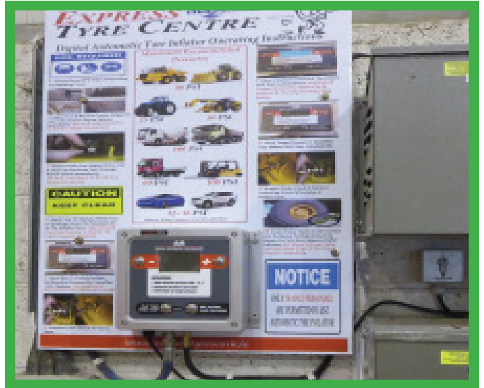
Best Practice example: To eliminate the risk of over inflation of tyres, tyre pressure is inputted remotely into a control unit. The 15 metre airline is then fitted to the vehicle (away from the control unit ) and a preset air pressure is used to inflate the tyre. Access to the control is restricted as users require access codes.
