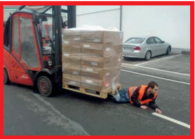
Reconstruction of a Serious accident – March 2015: Worker was struck by a forward moving forklift. Driver's view was restricted by load.
