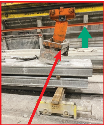
When the slab was lowered into position - the operator released the grabs / clamp and lifted the clamps higher upward to move them away from the next task.
