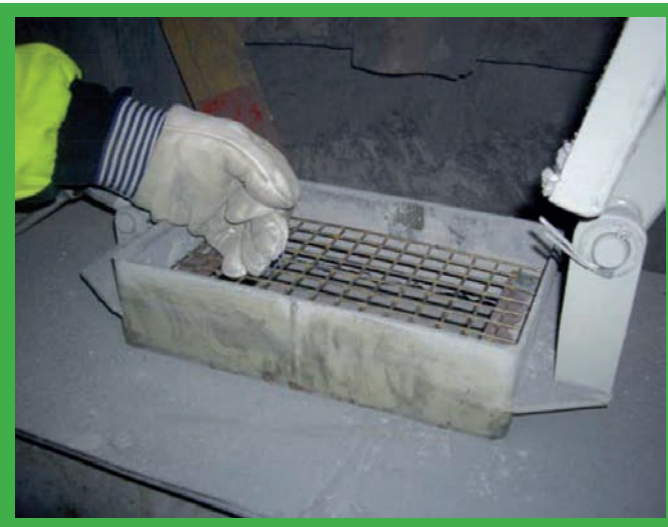
Inspection hatch (with secured grid) on a screw conveyor.
