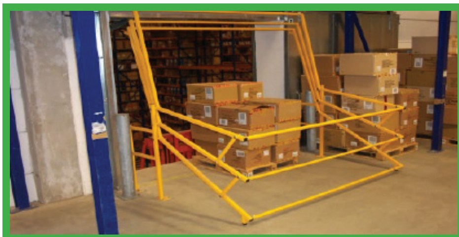
A revolving cage system which offers protection against falls.
